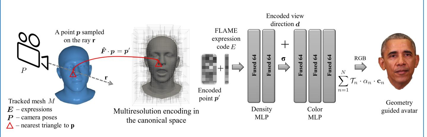
Tracker To get the precise geometry needed for accurate projection we used a tracker from MICA [Zielonka et al. 2022].
